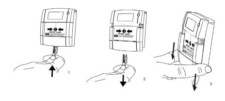
A test key is provided with each MCP to allow easy testing of the switch mechanism and wiring, without breaking the frangible element. The key is inserted into a slot in the base of the MCP, allowing the frangible element to drop away from the switch, thus activating it and registering an alarm at the CIE. Note: the key should not be left with the MCP after commissioning, but may be left inside the CIE for convenience.
